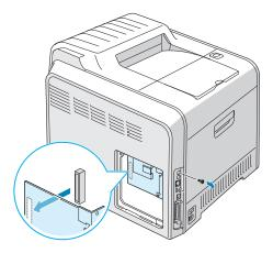
**5** Align the connector on the network interface card with the connector on the control board. Make sure that the jacks on the card go through the holes. Push the card firmly into the connector until it is completely inserted into place.
